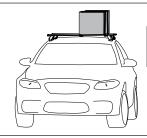
68kg load rating (Urban road) = 45kg load rating (Off road - 68kg / 1.5)
