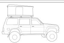
When these roof racks are to be used on a vehicle that is driven off sealed roads, the maximum roof rack load rating should be *divided* by 1.5. Do not forget to subtract 5kg from your maximum carrying capacity due to the weight of the crossbars and legs.
